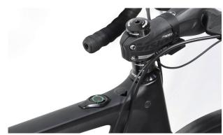
▲ The System features an integrated on-bike control.
