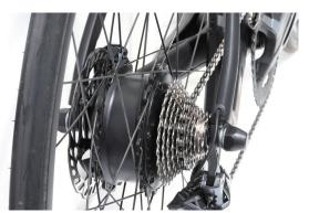
▲ The FSA System utilizes a rear hub electric assist drive
